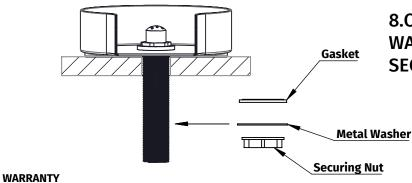
8.ONCE SHANK IS THROUGH SINK, SLIDE GASKET AND METAL WASHER THROUGH SHANK AND SECURE ASSEMBLY WITH SECURING NUT
