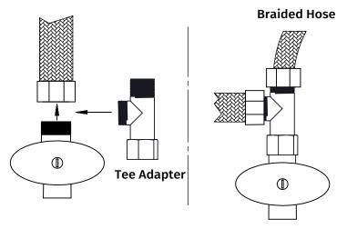
3.UNSCREW CURRENT SUPPLY CONNECTION HOSE AND SECURELY SCREW IN SUPPLIED TEE ADAPTER
